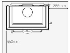
**HEARTH WIDTH:** Due to the side opening door on the Isotto Evo there must be a minimum of 300mm hearth clearance to the right of the fireplace.
